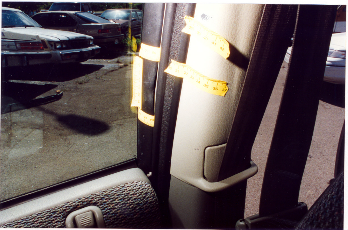
94. Close-up view of the rebound contact.
